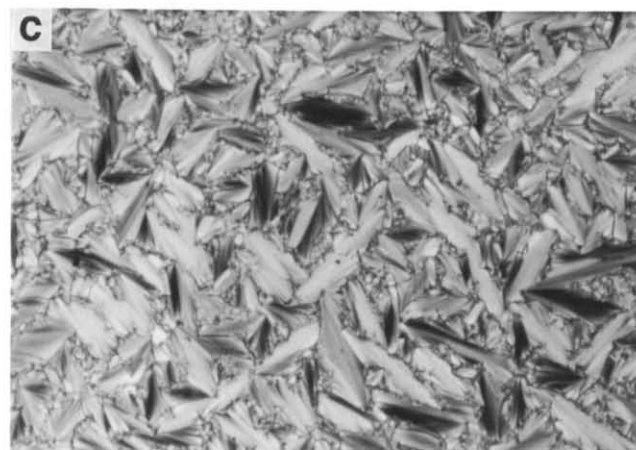
Figure 7 Representative optical polarized micrographs (100 \times ) of: (a) the n mesophase displayed by poly( 6-5 ) (d.p. = 24.4) at 105°C on the cooling scan; (b) the s A mesophase displayed by poly( 6-5 ) (d.p. = 24.4) at 70°C on the cooling scan; (c) the s A mesophase displayed by poly( 6-7 ) (d.p. = 26.4) at 120°C on the cooling scan
